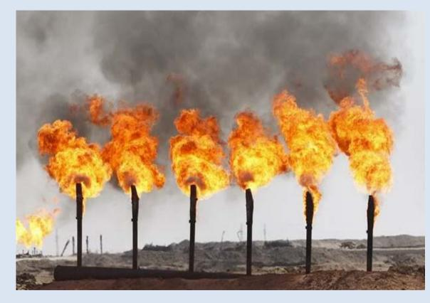
a) enormous waste of energy (the 20 billion m<sup>3</sup> flare gas burned every year only in Russia could be used to generate more than 8.5 billion MW )
